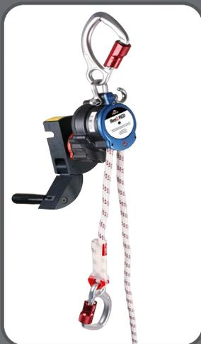
Device for rescuing or evacuating personnel from the Nacelle if the escape routes are blocked by fire. The device is fitted with a brake system that ensures that descending speed never exceeds 0.7m/sec (approx. half the normal walking speed). The low descend speed also helps to guarantee that the user has both hands free at all times. It is also approved for the descent of more than one person.
