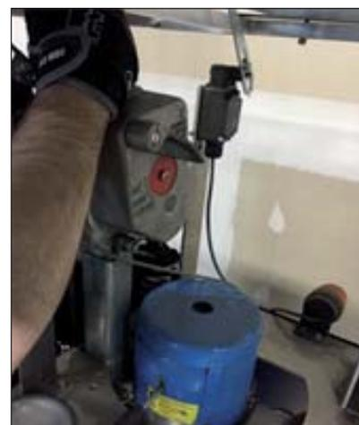
**Step 5** – If locked, reset the BlocStop to ensure the jaws are open by pulling downward on the reset lever. Move up the cabin lift 0,5 mts above the landing platform by pressing the up button on the pendant control.
