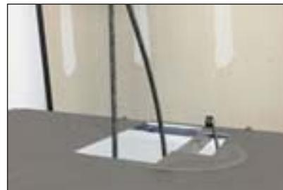
**Step 3** – With a gloved hand, push on the loop of wire so that it moves rapidly upwards through the BlocStop. The BlocStop should lock onto the drive wire.
